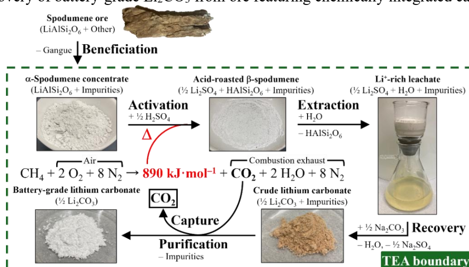
Figure 1. Recovery of battery-grade \text{Li}_2\text{CO}_3 from ore featuring chemically integrated capture of \text{CO}_2 . [2]
